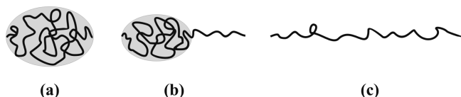
Figure 1. Conformation of stretched globule: prolate (ellipsoidal) (a), tadpole (b), and stretched chain (c).
